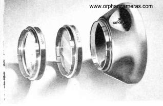
Voigtlander filters are available in both light and medium yellow. Focar attachments open up the field of close-up photography. The (#1) Focar permits working at distances from 17" to 32", while the (#2) can be used for close-ups from 12" to 17". The Voigtlander sunshade is a particularly useful accessory, serving to hold back extraneous rays.
