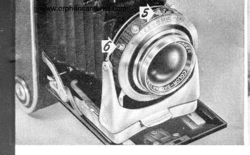
Compur Rapid shutter with delayed action and built-in flash Shutter speeds range from one second to 1/400th, in addition to bulb. If the photographer wishes to appear in the photograph, it is merely necessary to adjust the delayed action shutter release (#5). Between operation of the release and the opening of the shutter, about twelve seconds will elapse — time enough to take one's place in the group.
