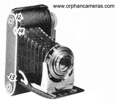
Speedy operation is another feature. The opening button (#14) is pressed and the Bessa is partly erected — the trigger shutter release, so cleverly concealed under the baseboard, emerges as if by magic — a downward motion on the baseboard, and presto the camera is ready for action.
